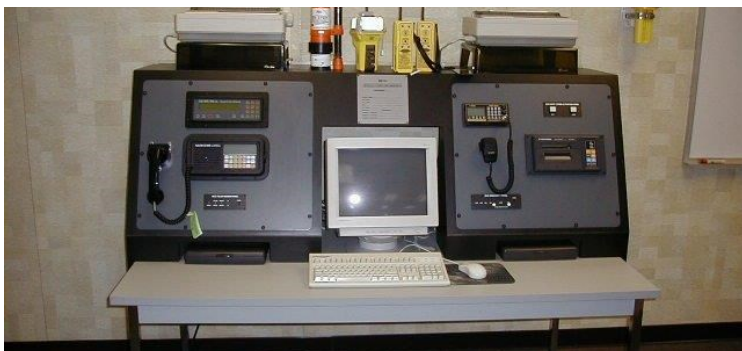
GMDSS Console comprised of modified real radios
