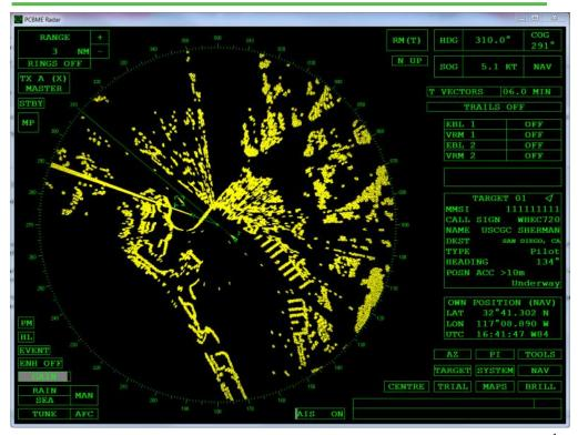
The PCBME ARPA Radar Emulator models the Sperry BridgeMaster-E<sup>1</sup> Radar Display and is one of many radar products in the Buffalo Computer Graphics' (BCG) family of successful PC-based simulators. It is a powerful, low-cost training tool to familiarize a student with the use of a real ARPA radar for ship navigation and collision avoidance.
