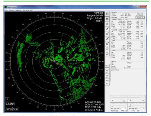
The PCRadar is an established product in the Buffalo Computer Graphics' (BCG) family of successful PC-based radar emulators. PCRadar is a Windows-based application which emulates a generic ARPA radar display on a PC monitor. It is a powerful training tool to familiarize a student with the use of radar for ship navigation and collision avoidance.
